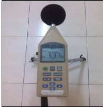
Rajah 2 Meter aras bunyi iaitu Integrating Sound Level Datalogger Model 407780 Extech Instrument
