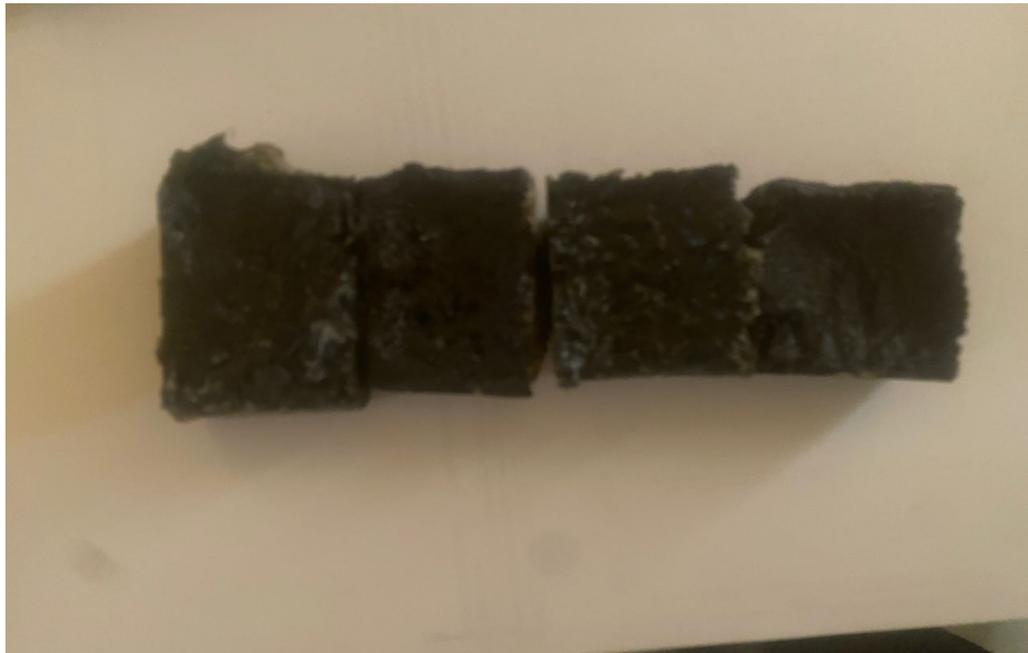
**Figure 4:** Fabricated Sand Reinforced Plastic Concrete Samples
