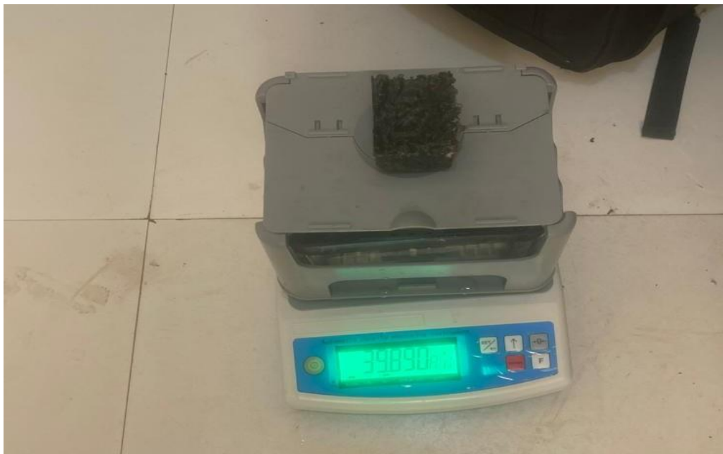
Figure 2: Density Measurement Procedure
