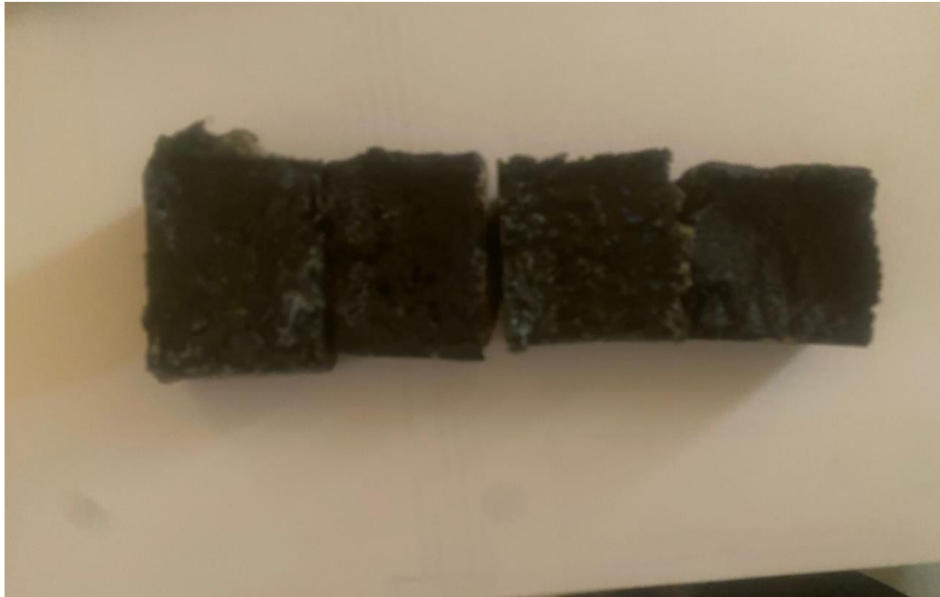
Figure 4: Fabricated Sand Reenforced Plastic Concrete Samples
