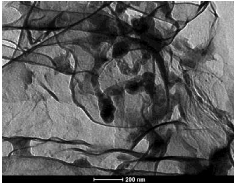
Figure 1 TEM images of reduced graphene oxide
