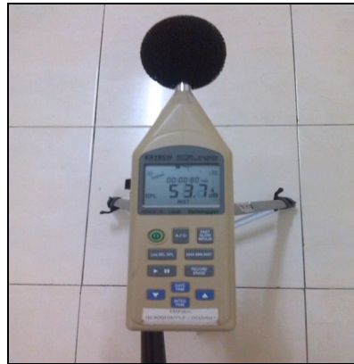
Rajah 2 Meter aras bunyi ( Integrating sound level datalogger Model 407780 Extech Instrument )
