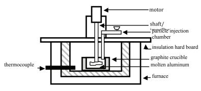
Figure 2 Schematic of stirring mechanism
