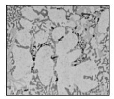
Figure 1 Microstructure of Mg<sub>2</sub>Si in alloy AA332-F(ASM International, 1992)
