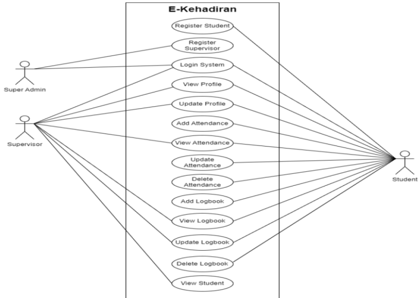
Figure 2: Use case diagram of the E-Kehadiran system
