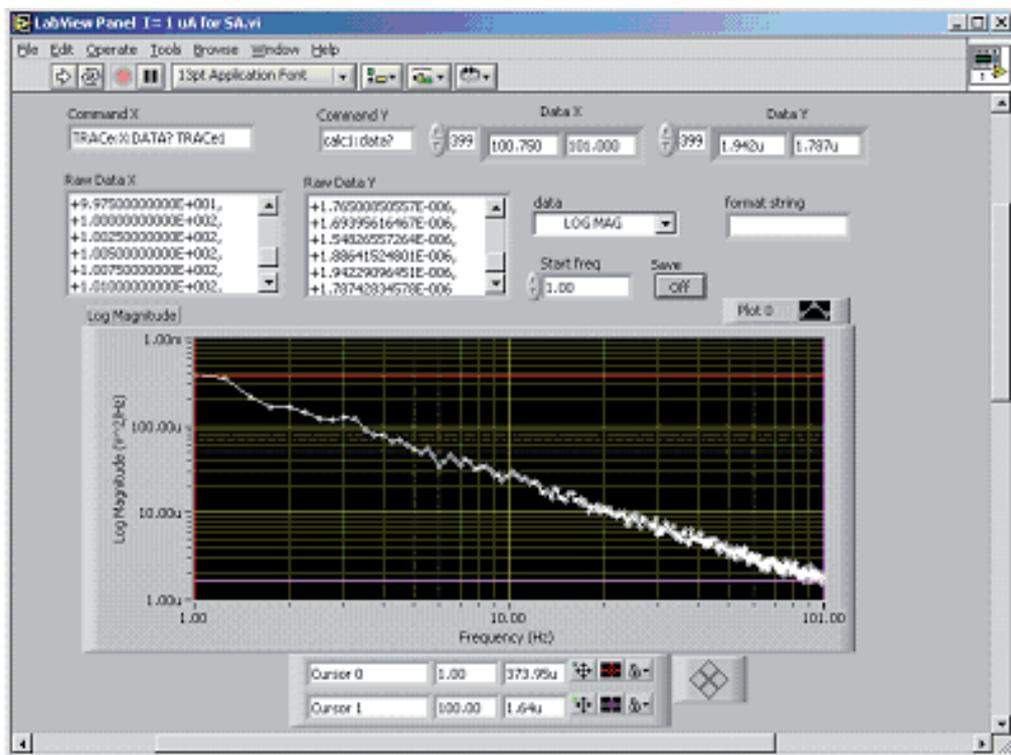
Figure 3 LabView panel window for acquiring PSDs data.
