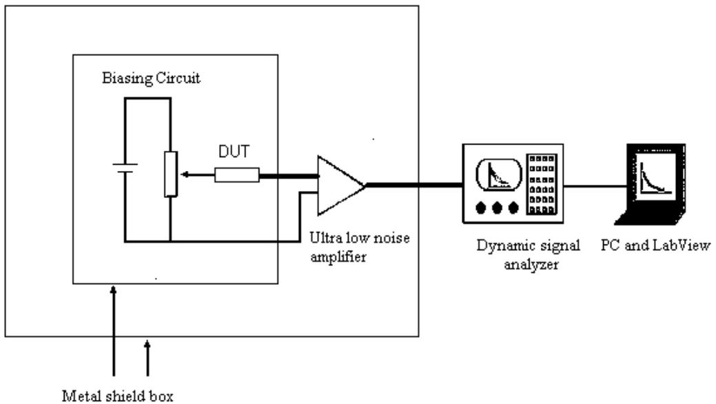
**Figure 1** Schematic diagram of the experimental setup for noise measurement
