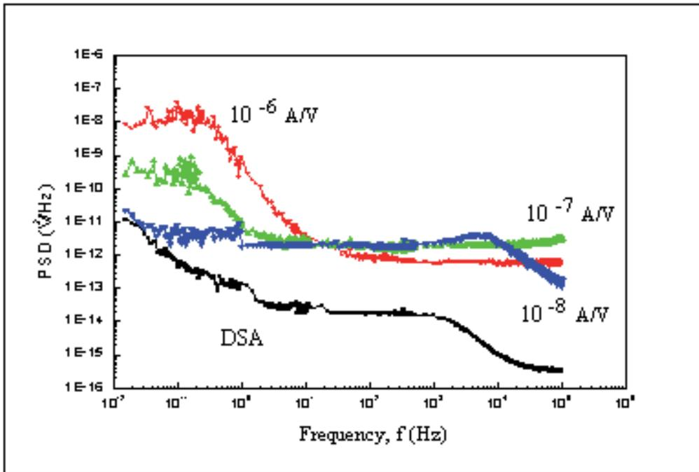
Figure 2 Background voltage noise power spectral density of transimpedance amplifier and dynamic signal analyzer.
