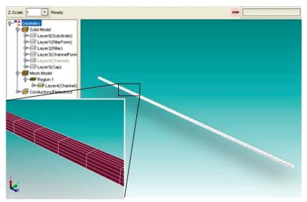
Figure 4 Meshing model of microchannel in MemCFD
