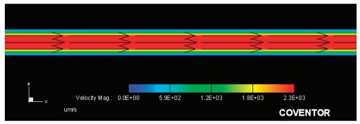
Figure 9 The blood velocity for pressure difference 1 kPa
