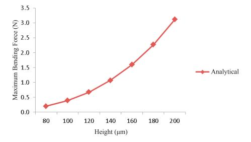
Figure 8 Maximum bending force with difference height
