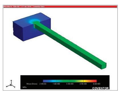
Figure 5 The distribution stress on the microneedle
