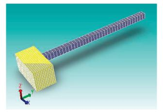
Figure 2 3D meshing of the microneedle model in CoventorWare
