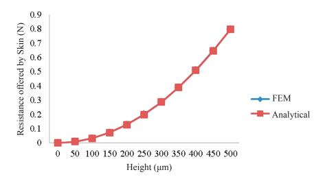
Figure 6 Resistance offered by skin with difference height
