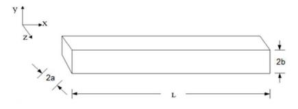
Figure 3 Model of rectangular duct for microchannel
