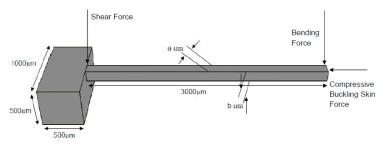
Figure 1 The various force acting on the microneedle
