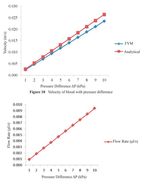
Figure 11 Flow rate of blood inside microchannel for difference pressure difference
