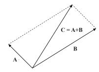
Figure 1 A graphical representation of vector addition. Vector C is the vector sum of vectors A and B
