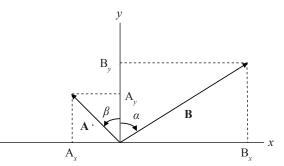
Figure 2 Decomposition of vector A and B into their respective components along coordinate axes
