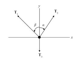
Figure 3 A free body diagram showing the forces acting on the knot of the strings
