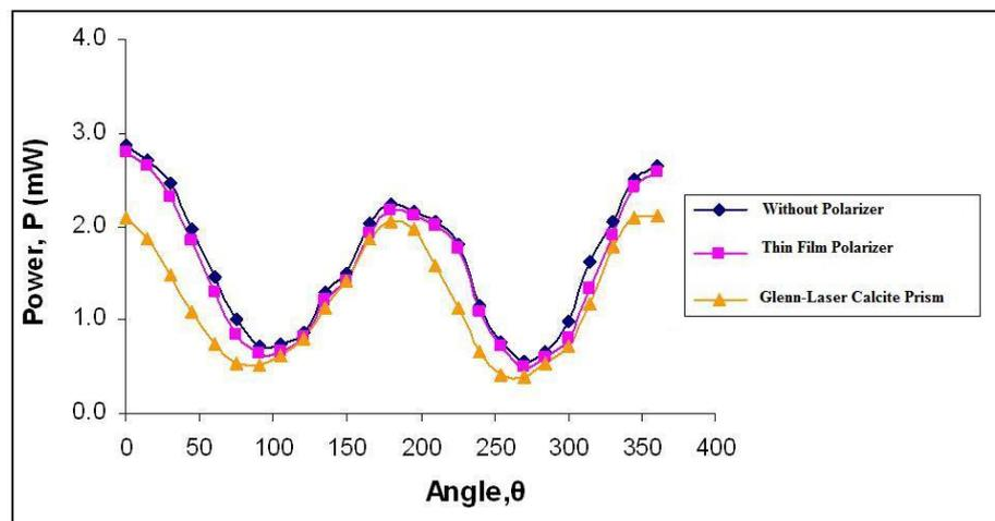
**Figure 4** The polarization profile of He-Ne beam
