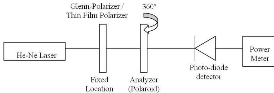
**Figure 3** Setup for testing the polarization purity and state of high-energy polarizer
