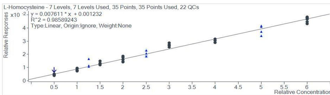
**Figure 2.** The linearity of the calibration levels with 3 QC levels
