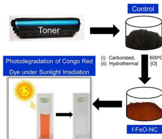
Figure 3. Diagram illustrating the separation of the functionalized version (f-FeO-NC) from the control (waste black toner ink) and its application to the degradation of the poisonous Congo red dye in the presence of natural sunlight (Saini et al., 2019).
